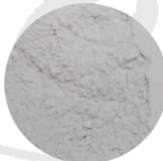
Use to remove grease or stains from glass surfaces. This pumice creates an excellent pre-polish on glass. Use with cork belts, wheels, or discs. Can be applied with wet rag, or felt block.
