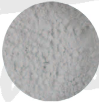
A 99% pure micro-alumina powder, this polish is great for polishing petrified wood, agate, rhodocrosite, jade and other hard stones. Approximately 2-3 microns and a 9 on the Mohs scale (compares with Tin Oxide).
