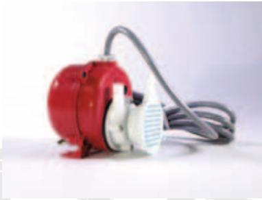
Covington's Submersible Pump will pump 200 gallons per hour at 1-foot or 105 gallons per hour at 5-feet.
