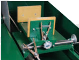
This book-end type vise holds work pieces of any shape tightly, but quick-release feature allows an easy, no-bind return. The steel jaw tongue contacts the full length of the vise, holding the jaw square so it can't bind. The end grips have a hardwood facing. A cross shaft is included with each vise.
