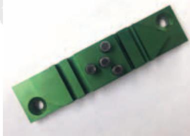
Covington's Jewelry Wire Bender is machined out of a solid piece of aluminum. It features two (2) mounting holes, four (4) removable dowel pins that assist in making almost any design, and a green anodized coating.
