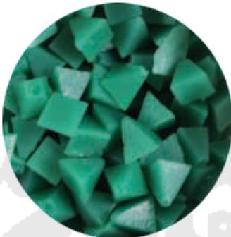
1/4" plastic media used wet on all precious metals for cut down prior to burnishing with steel shot. This is a fast cutting media that produces an excellent finish. The plastic pyramids are made with a 400-grit quartz abrasive embedded inside.
