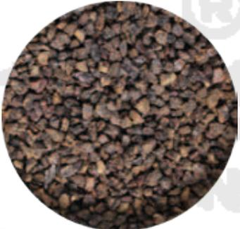
An excellent aid to grinding and polishing in a vibrating or rolling tumbler. The small size aids in reaching hard-to-get areas. Use 1/4-cup of garnet sand per quart of rocks. Use the mixture from rough grind through polish. 8/12 mesh.
