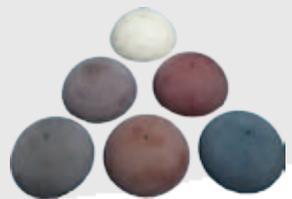
Resin Bonded Diamond Domes are an excellent choice for working bottles and inside curves. These domes are approximately 4" at base and 2-1/2" in height. Standard sizes available are: 1"-14 female or male, 5/8"-11 female or male, and 1/2"-20 female or male. All domes are special order and will be shipped once manufactured, alternate sizes can be manufactured but will take an additional week. All domes are available in 100g, 220g, 325g, 600g, & 1,200g, and left or right hand threads.
