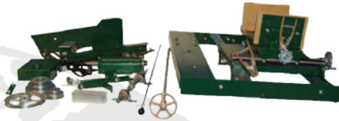
The Carriage Slab Saw Kit is a "build-your-own" style unit that requires the user to construct a tank. This kit comes complete with a saw frame, carriage and vise assembly, arbor, blade guard, rock catcher, and power feed assembly. The carriage assembly ships mounted on the guide ways within the saw frame.
