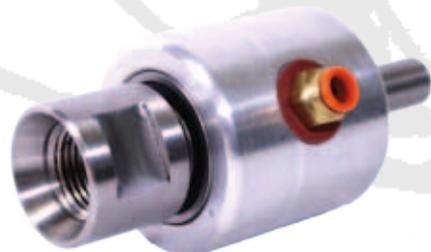
Covington's new Water Feed Drill Assembly features a through shaft water feed that provides water directly to the core drill while flushing debris away from the work area. Never use a household water source; use a submersible pump to supply water to the system. Available in two options: 3/4"-12 female threading for brass core drill inserts, or with collet for a variety of core drill shank sizes.
