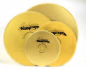
Covington's Gold Series Diamond Blades are excellent quality, commercial grade blades, designed for lapidary work. More diamonds in the notched rim and a stiffer core make this blade cut faster and maintain a longer use life. While this blade was designed for use on hard materials like agates, geodes, and petrified wood, it will cut soft materials such as glass superbly. The Gold Series blades are a great low cost choice. \*Please specify arbor size when ordering, 1/2", 5/8", 3/4", or 1".
