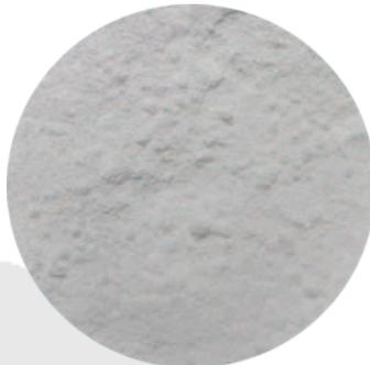
A .3 micron alumina powder that is 99.98% pure aluminum oxide and a 9 on the Mohs scale. Linde 'A' will polish almost any gemstone.
