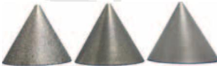
Nickel Bonded Diamond Cones are an excellent choice for working bottles and inside curves. These cones are approximately 3" at base and 3" in height. Standard sizes available are: 1"-14 female and 5/8"-11 female. Cones are available in Coarse (100g), Medium (220g), and Fine (600g). All cones include a 3/16" center hole for through-shaft water systems.
