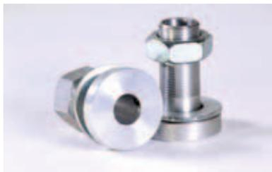
Large Shaft Adapters are a 1"-14 with a left or right hand nut thread. Each has 2" inside backing stop for wheel or buff mount. Adapters come in 1/2", 5/8", or 3/4" bore. \*Please specify bore size and thread.
