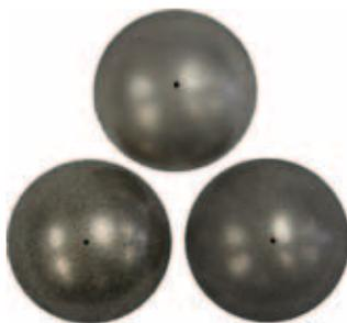
Nickel Bonded Diamond Domes are an excellent choice for working bottles and inside curves. These domes are approximately 3-7/8" at base and 1-1/2" in height. Standard sizes available are: 1"-14 female and 5/8"-11 female. Cones are available in Coarse (100g), Medium (220g), and Fine (600g). All domes include a 3/16" center hole for through-shaft water systems.
