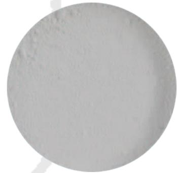
A 99% pure micro alumina powder, this polish is excellent for achieving a super-fine polish on all hard and soft stones. Particle size is approximately .5 microns and a 9 on the Mohs scale (compares with Linde 'A' Polish).
