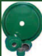
The Sphere Cutting Tool Kit will make spheres from 1-1/4" to 4" in size. Cups have a 1"-8RH threaded bore to fit horizontal lap arbors. This kit consists of a special splash guard and one (1) each: 1", 1-3/8", and 2-3/8" cutter cups. Sphere cutting on this unit is simple, just hold the rough sphere with a gloved hand and grind it on the proper size sphere cutter cup.
