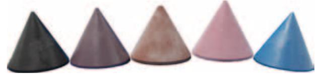
Resin Bonded Diamond Cones are an excellent choice for working bottles and inside curves. These cones are approximately 3" at base and 3" in height. Standard sizes available are: 1"-14 female or male, 5/8"-11 female or male, and 1/2"-20 female or male. All cones are special order and will be shipped once manufactured, alternate sizes can be manufactured but will take an additional week. All cones are available in 100g, 220g, 325g, 600g, & 1,200g, and left or right hand threads.
