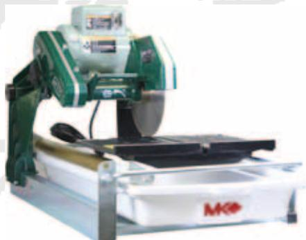
The Covington-MK saw has been modified especially for glass. Whether you are cutting Borosilicate, Soft Glass, Pattern bars, or even bottles our Covington modified MK saw will do the trick. We have modified the RPM's of the tile saw and slowed it down from 3450 RPM's to 2500 RPM so the glass does not get "hammered". We include our Ultimate Glass Blade (a \$150.00 Value) with each saw to provide you with everything you need to get nice clean, virtually chip free cuts. (Available in 110v or 220v)
